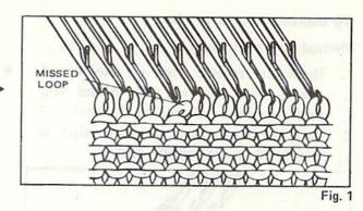
■ Insert a transfer tool into the loop just below the missed loop. Hook it on the empty latch needle together with the missed loop.
