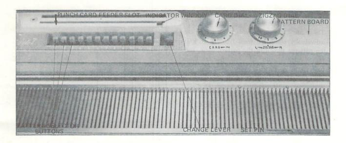
PATTERN SELECTOR BUTTONS · Used for Manual needle selecting
