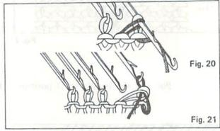
Transfer this stitch to the next inside needle, and push the empty needle to A position.
