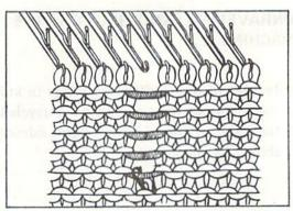
Push the latch needle tool through the knitted fabric from the back again forcing the loop on the hook back over the latch and onto the latch needle tool shaft. Again withdraw the tool picking up the cross thread above it and continue until all the stitches are knitted.
