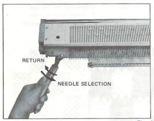
■ Turn the needle selector lever as far as it will go and return it to the original position completely.
