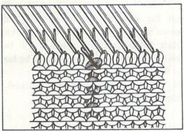
Unhook the latch needle tool, and pick up the loop with a transfer tool from the front and hook it on the needle.
